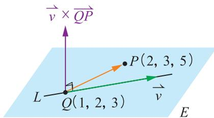
$$\vec{v} \times \vec{QP} = \left( \begin{vmatrix} 3 & 2 \\ 1 & 2 \end{vmatrix}, \begin{vmatrix} 2 & 2 \\ 2 & 1 \end{vmatrix}, \begin{vmatrix} 2 & 3 \\ 1 & 1 \end{vmatrix} \right) = (4, -2, -1),$$
